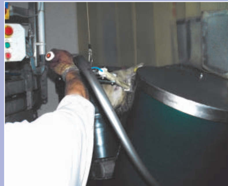
Stunning device FBT 2000 A with pneumatic tong FBTZ in combination with restrainer for the stunning of sheep
