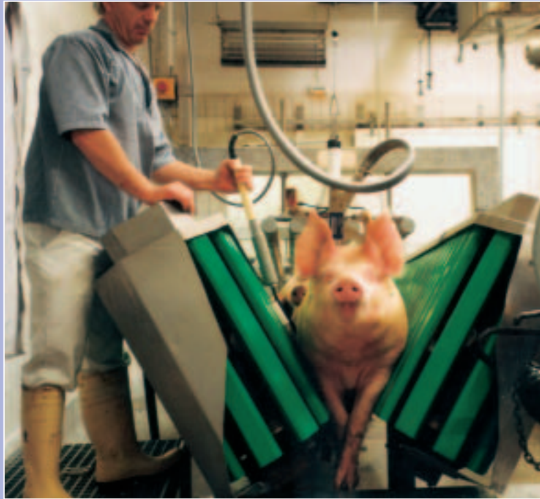
Stunning device FBT 2000 A in combination with restrainer, pneumatic stunning tong FBTZ and manual heart electrode
