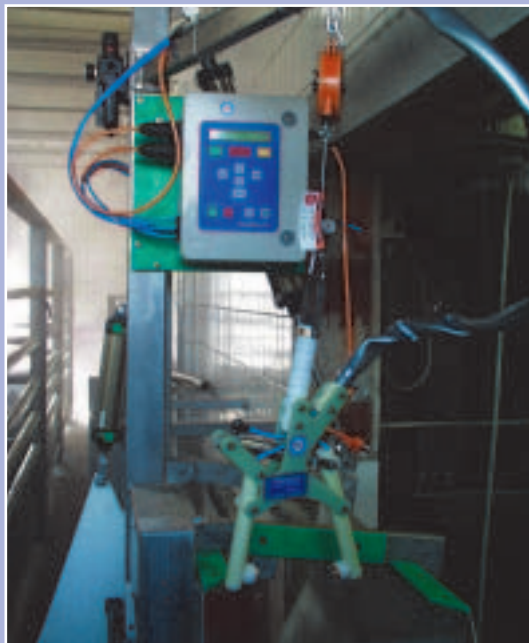
Stunning device FBT 2000 A, in combination with various stunning traps and pneumatic tong FBTZ
